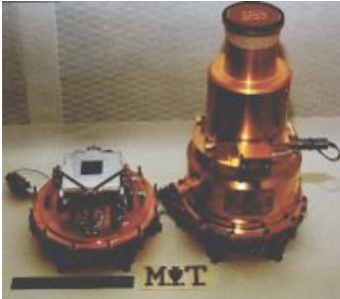
Solid State Imaging Spectrometer (SIS) for the ASCA Satellite (...First photon-counting CCD array flown in space)
