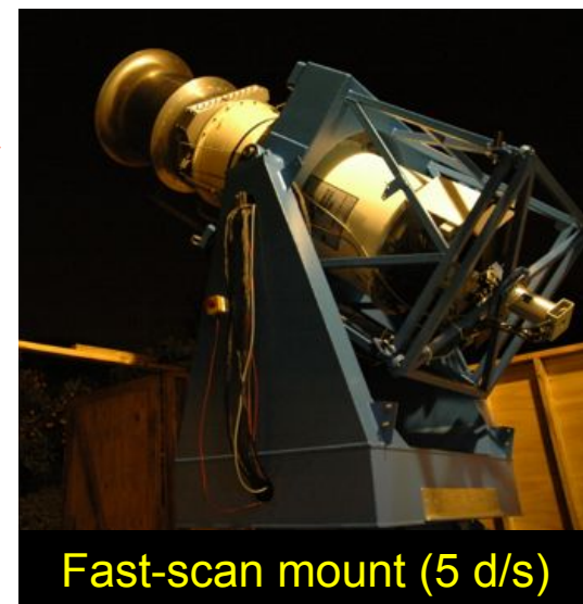
Telescope: 30 cm wide-field refractor, all optics at 4 K
